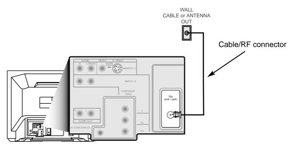
1) Connect an RF cable out from the wall outlet in to the RF Input on the back of the TV.
